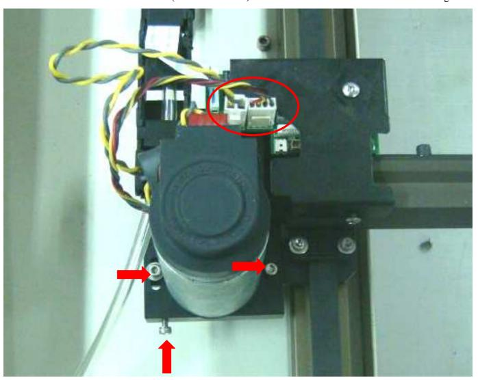
3-1. Dismount 2 screws of x motor cover and 2 screws of carriage cover.
