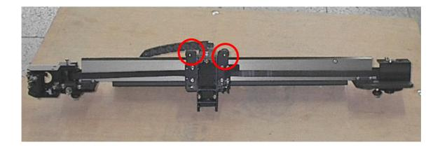
2. On the front of lens carriage, there are four screws for x axis belt retainer (see red circles below. Two screws on the right and two screws on the left). On the back of lens carriage, the location of the belt retainer can be seen. Loosen the belt retainer, the lens carriage can remove from x axis belt.
