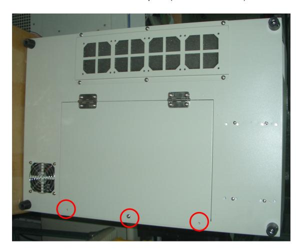
2. Dismount 7 screws (see red circles below) and remove all cables connecting to main board and can change new main board.
